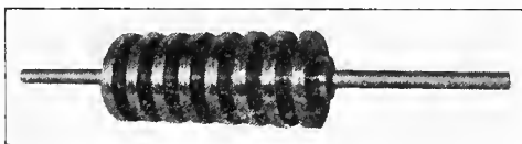
Fig. 45. The discs of a Disc Continuous Freezer.
